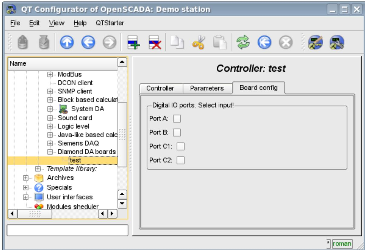
Fig.2. Tab of configuration of digital inputs / outputs ports.
