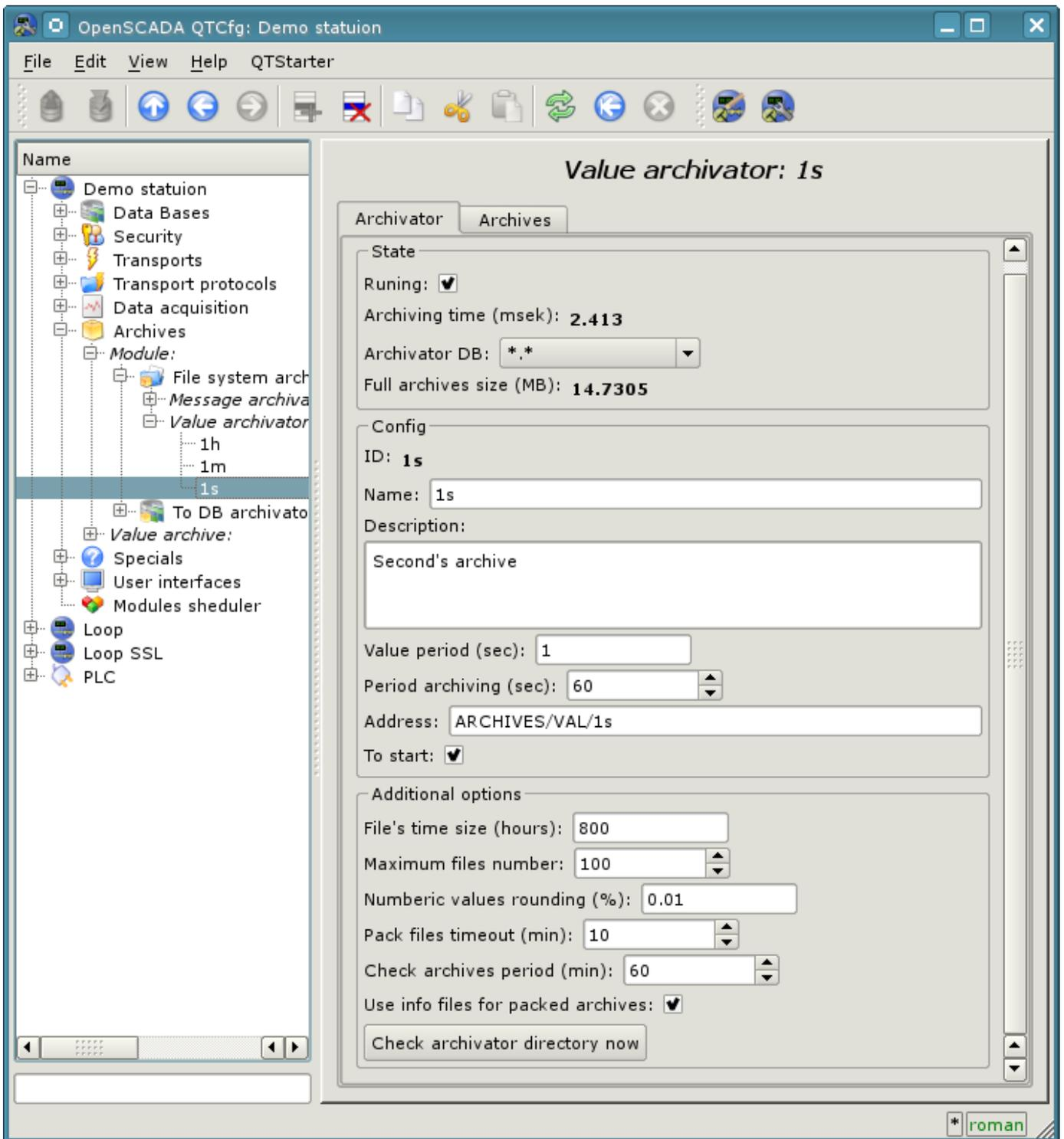
Fig.3. Additional settings of an archiving process of values by module FSArch.
