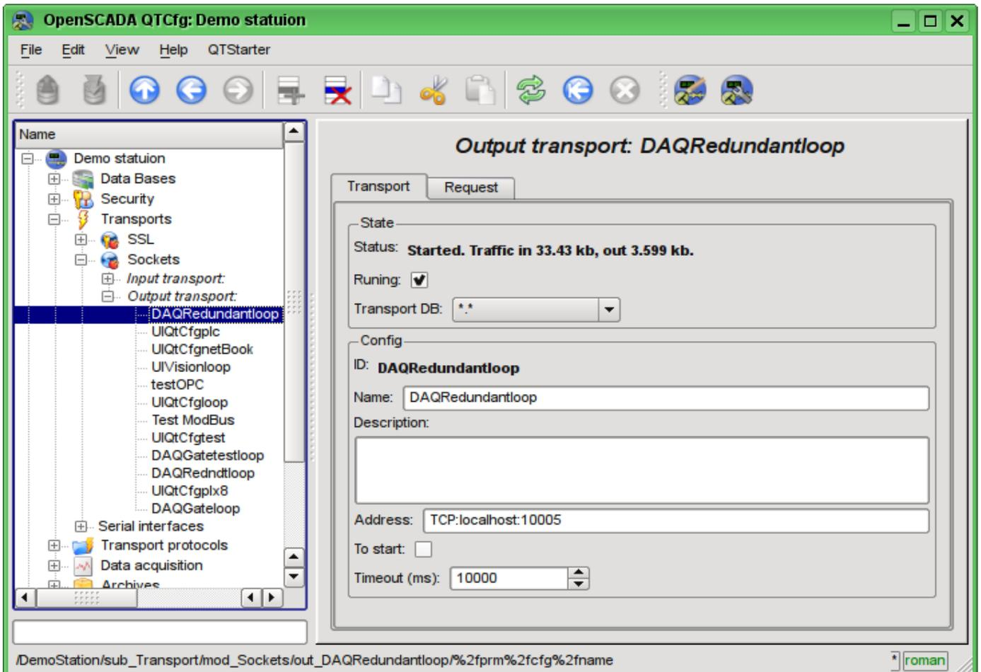
Fig. 4.3e. Tab "Transport" of the page of outgoing transport of module of subsystem "Transports".
