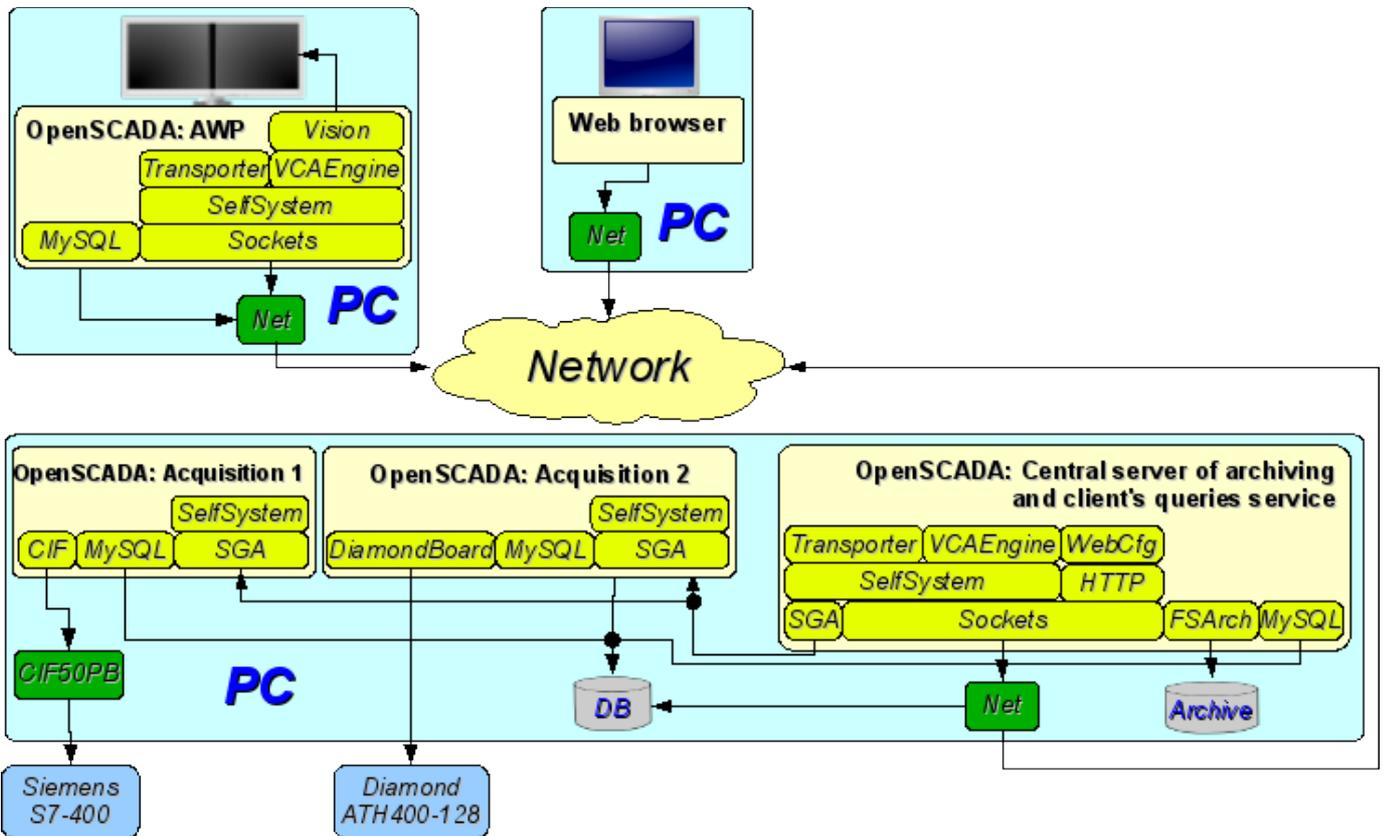
Fig. 3.8. The steady, allocated configuration.
