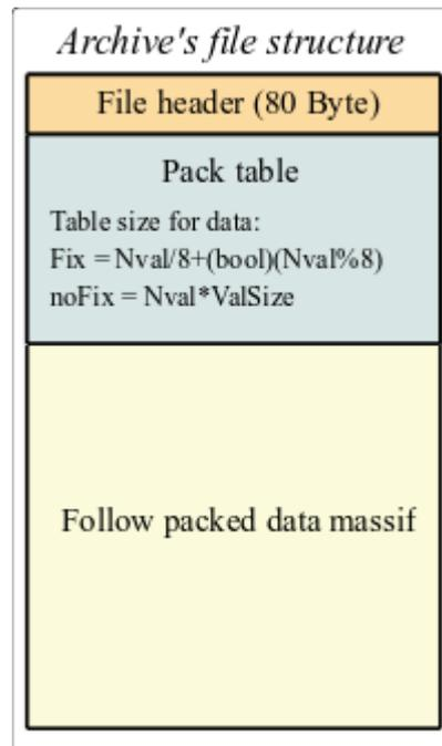
Fig. 4. The overall structure of the value archive.
