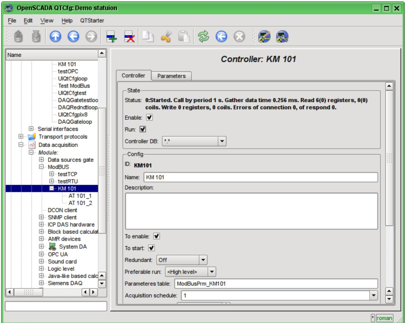
Fig. 4.1.7. The page of the controller's object if the exchange with the physical controller is successful.
