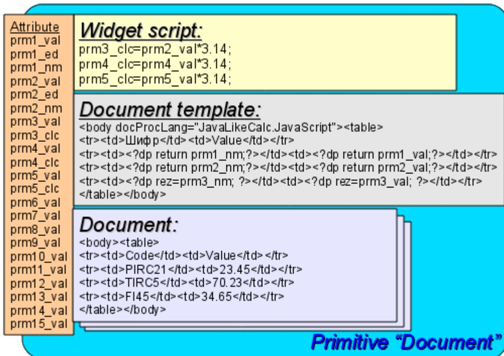
Fig. 3.8.7.a The block diagram of the primitive "Document".
