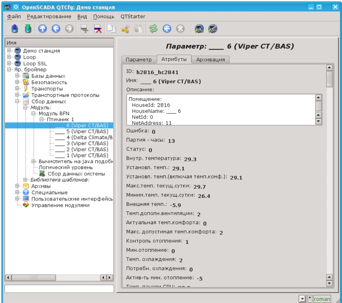
Fig.3. The "Attributes" tab of the poultry house computer's parameter.
