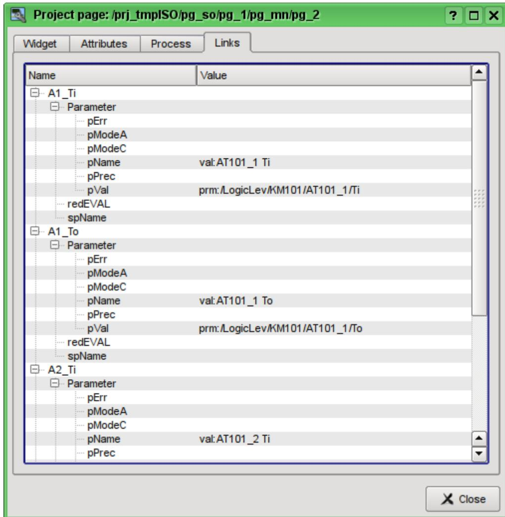
Fig. 5.2.5. The "Links" tab of dialog of editing the properties of the mnemonic scheme.
