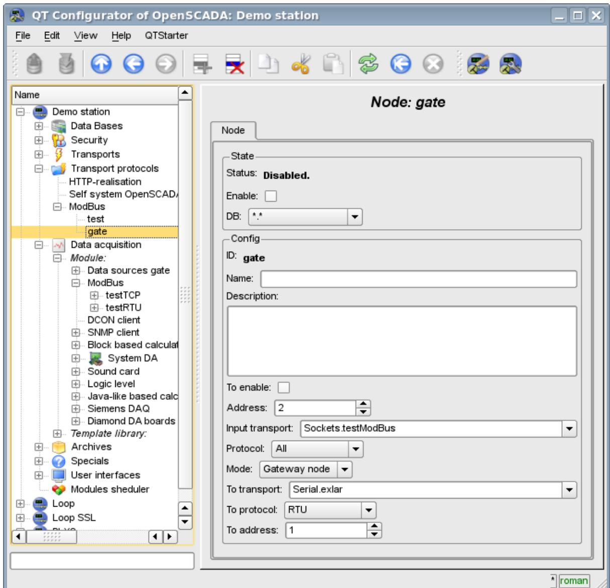
Fig.5. The tab “Node” of the configuration page of the node of the protocol in the “Gateway of the node”
