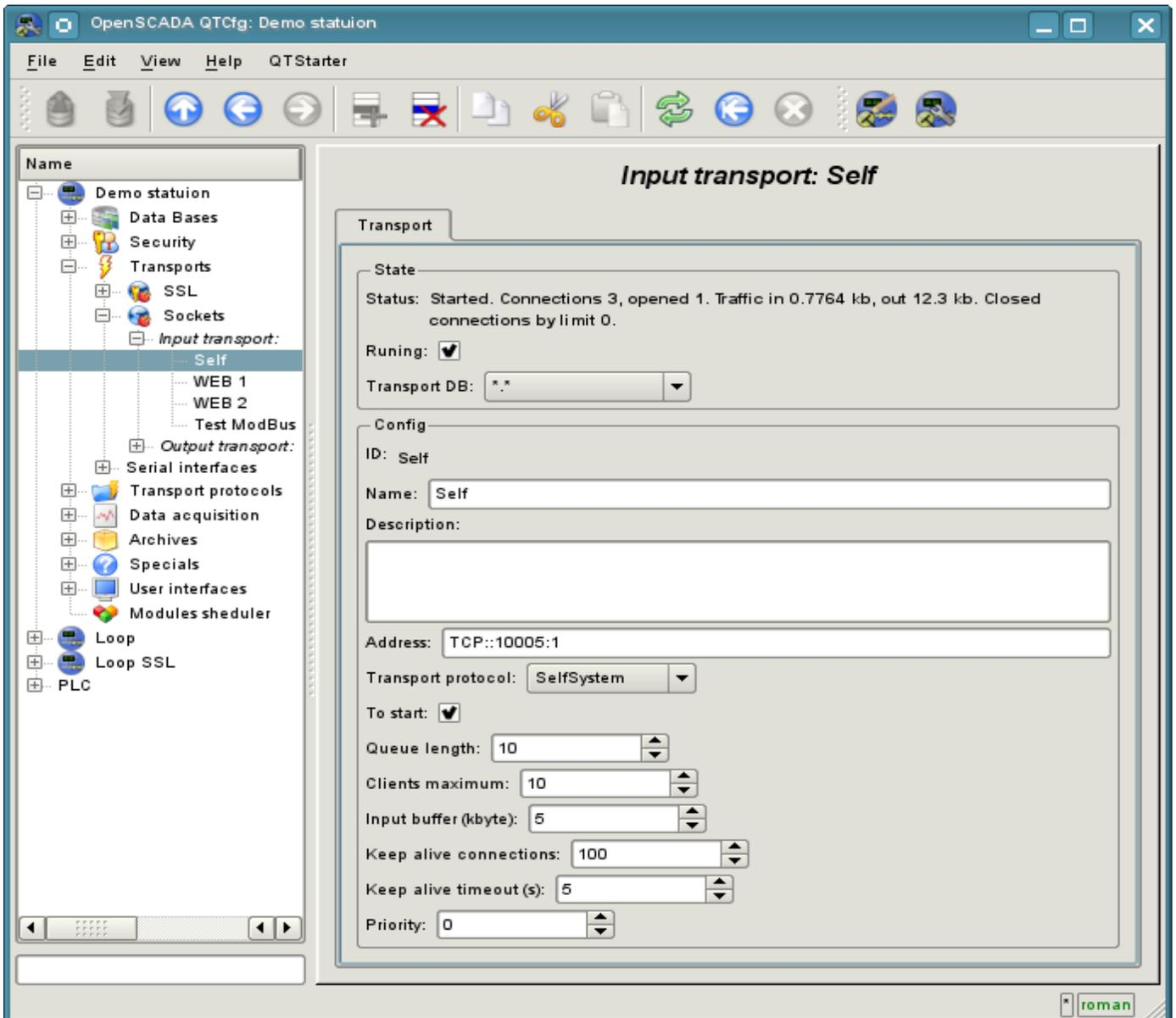
Fig.1. Configuration dialog of the incoming socket.
