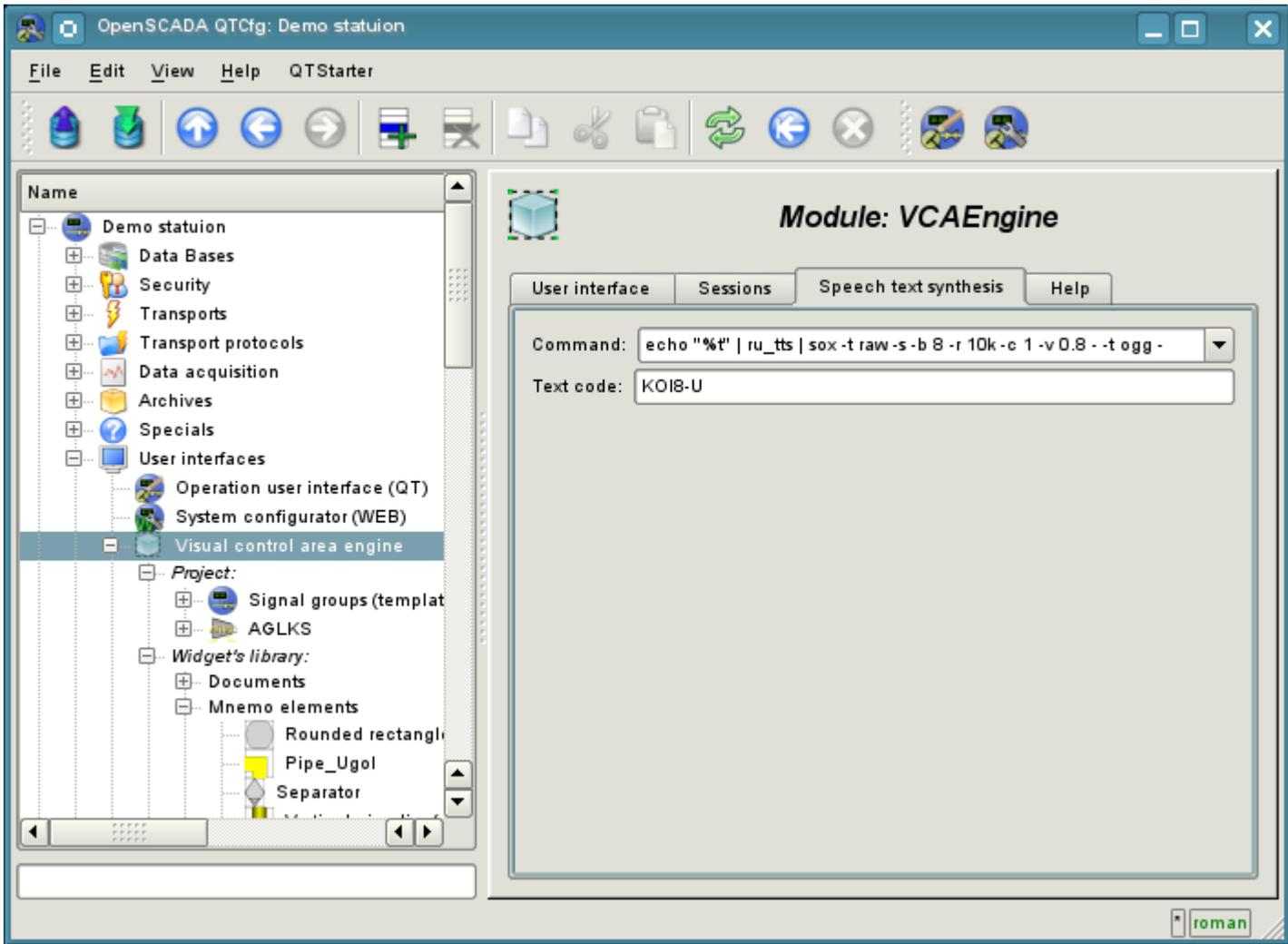
Fig.4.3 The inset for speech synthesis engine configuration.
