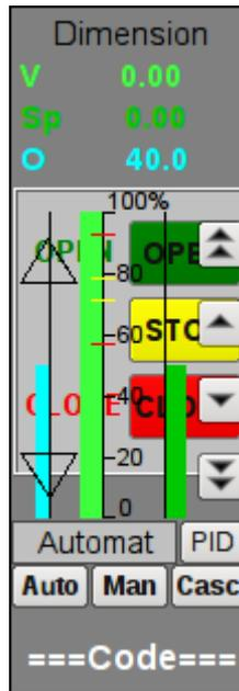
Fig.3. "Element cadr" widget in the development mode.
