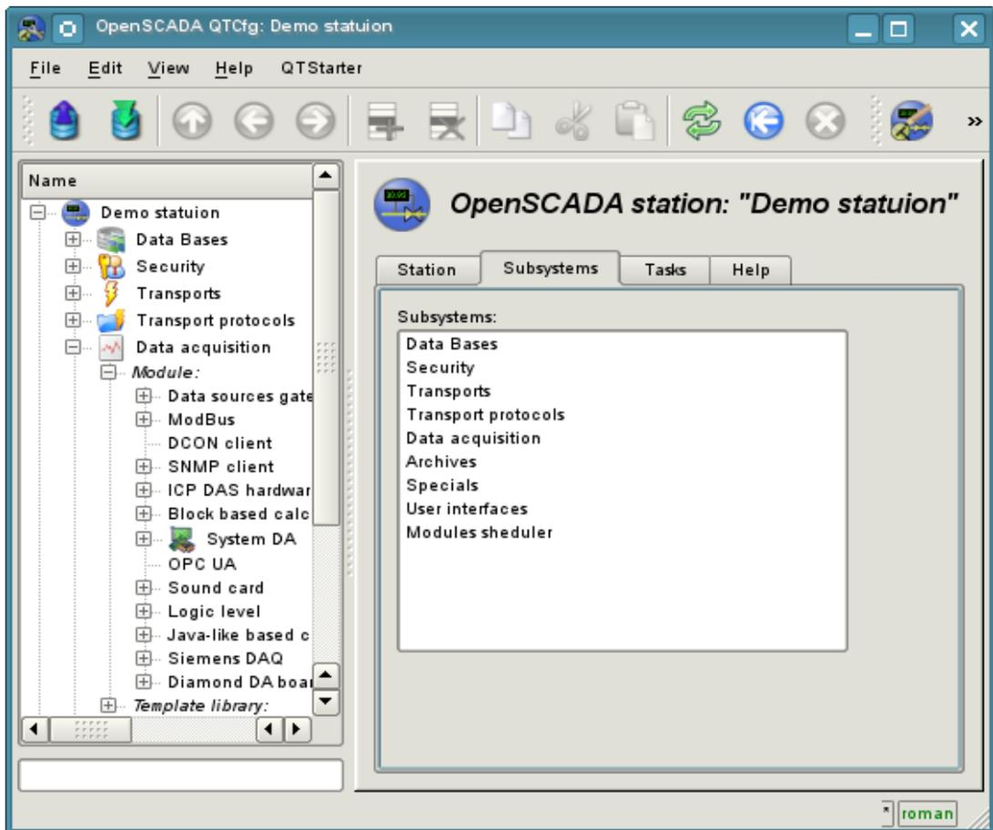
Fig 4b. "Subsystems" tab of the main page of the configuration of the station.
