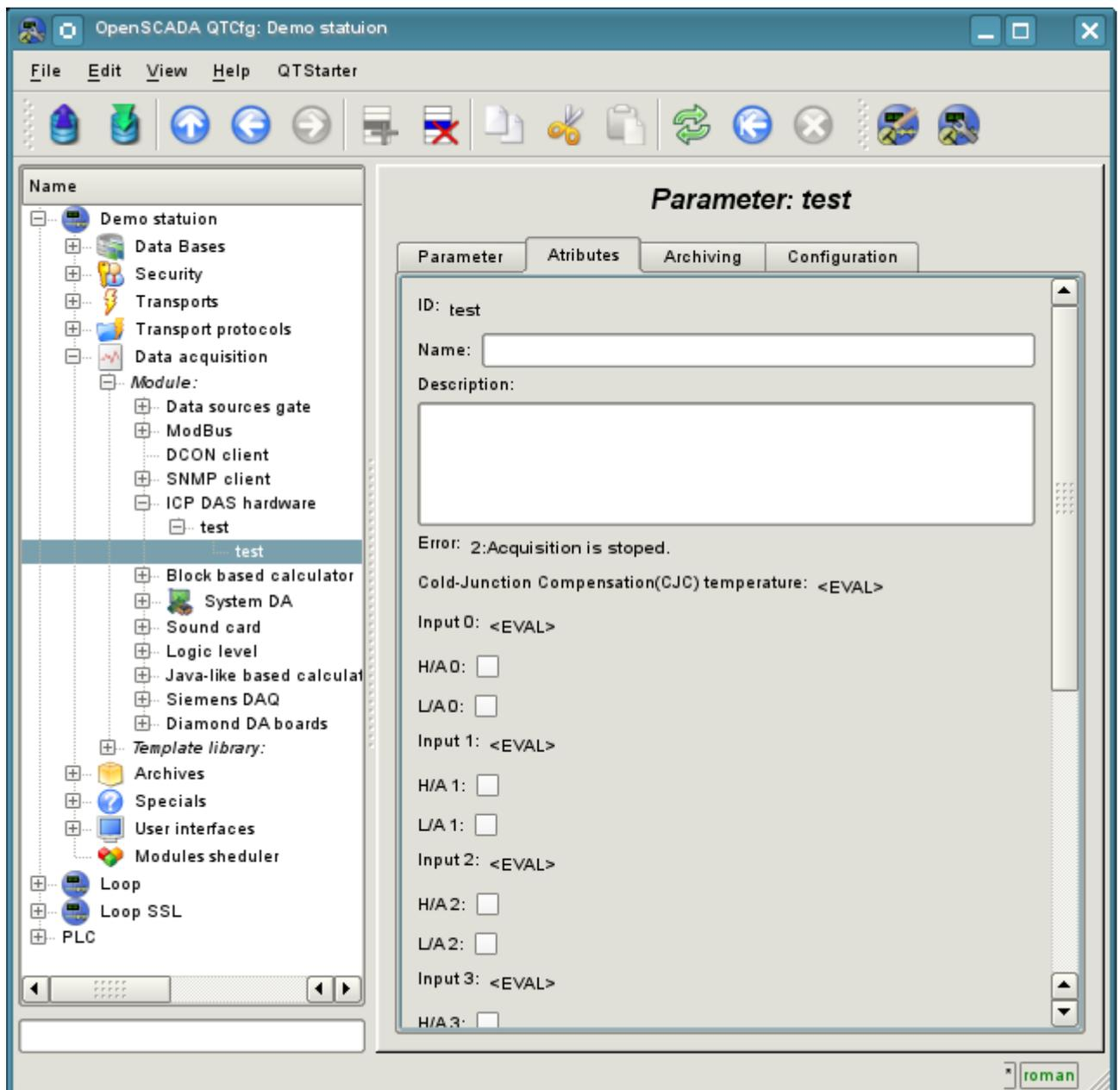
Fig.3. Tab of the attributes of the parameter.
