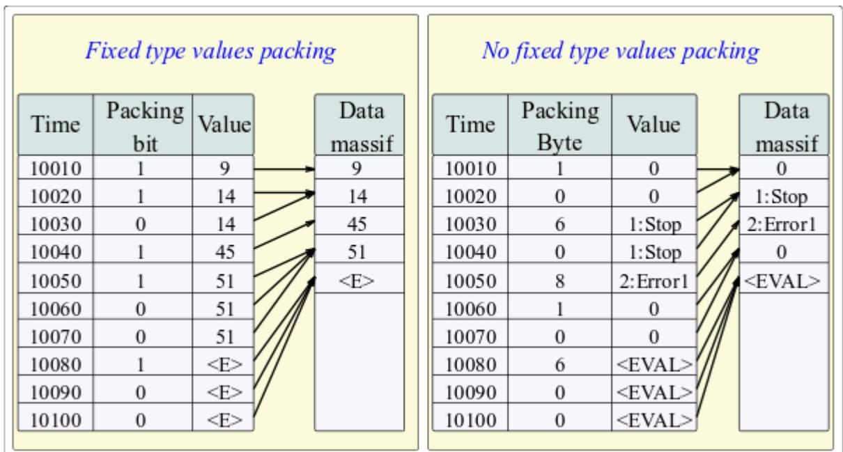
Fig. 5. The mechanism of follow packaging of values.
