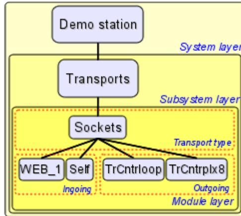
Fig. 4.3a. The hierarchical structure of subsystems "Transports".
