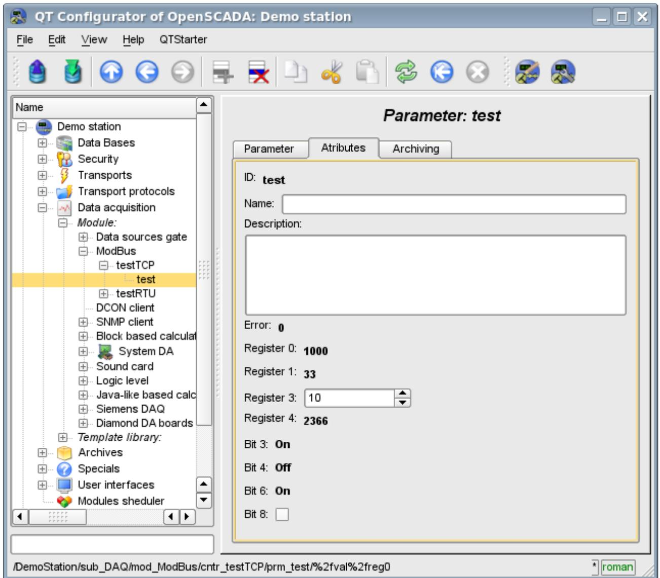
Fig.10. Tab of the attributes of the parameter.
