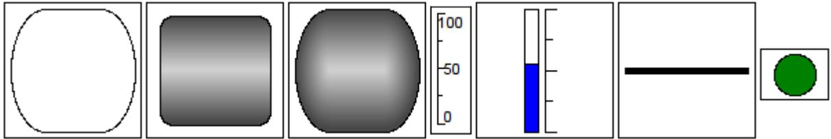
Fig.4. Elements from left to right and top to bottom: "Rounded rectangle", "Rounded rectangle (variant 2)", "Rounded rectangle(valuable)", "Scale", "Level", "Line", "Alarming".
