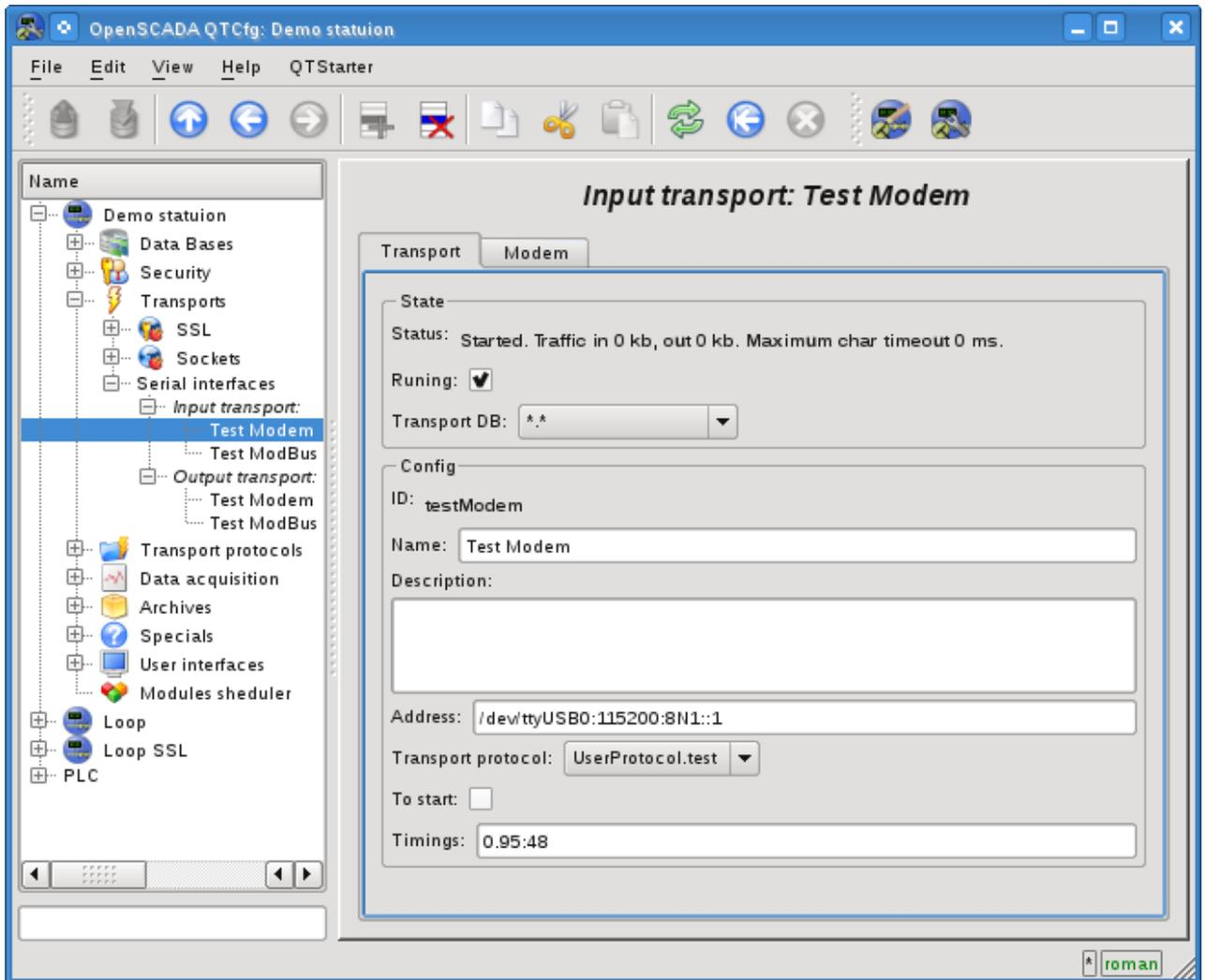
Fig.1. Configuration dialog of the incoming serial interface.
