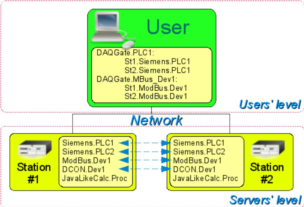
Fig.1. Horizontal and vertical redundancy.
