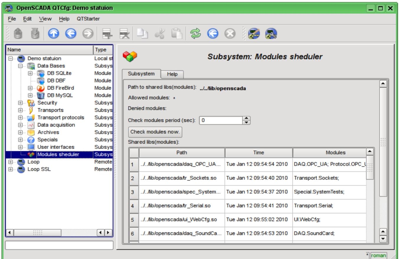
Fig. 4.9a. The main configuration tab of subsystem "Modules scheduler".
