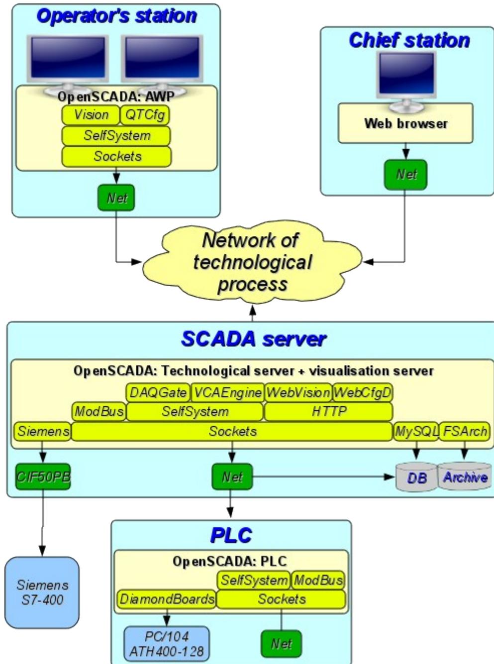
Fig. 1. OpenSCADA system's roles
