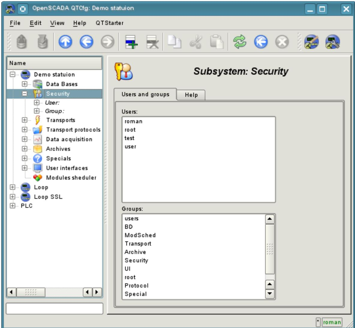
Fig. 4.2a. Tab "Users and Groups" of the root page of the subsystem "Security".
