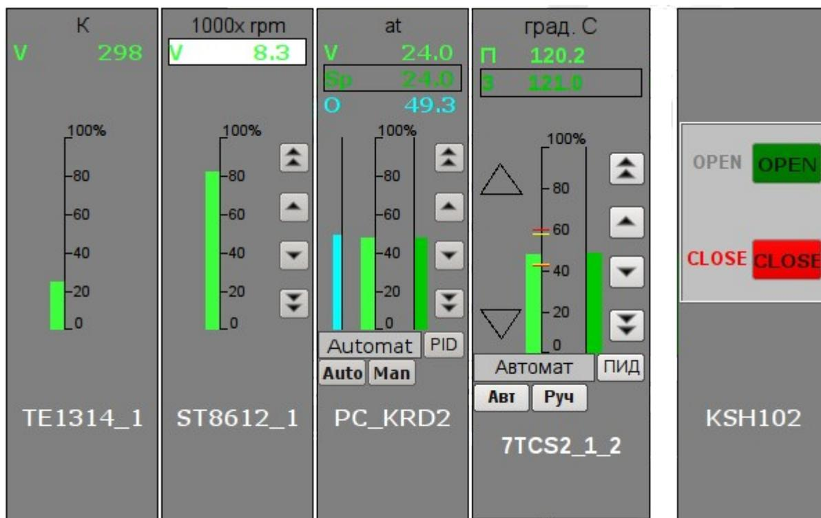
Fig.4. "Element cadr" widget in the runtime mode.
