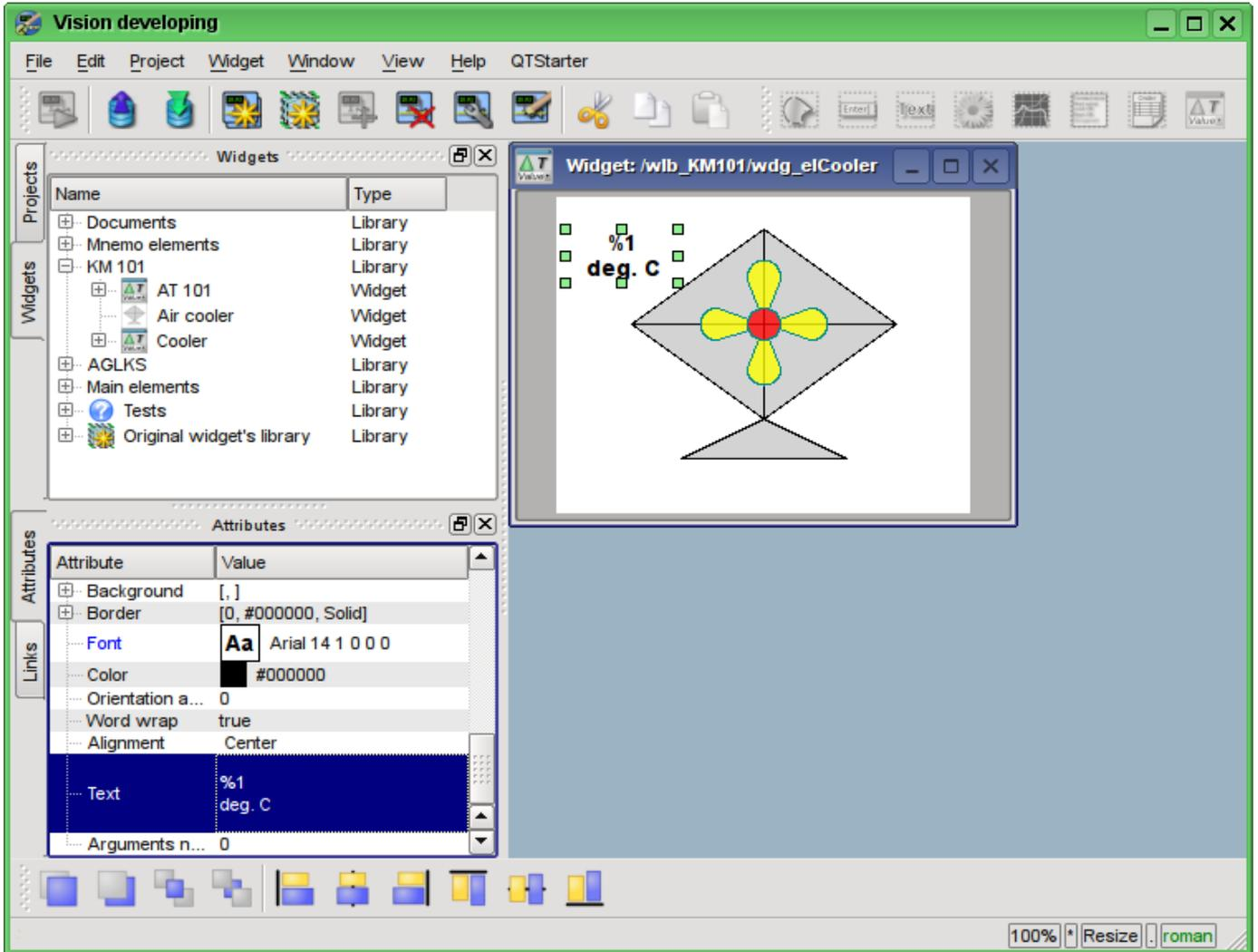
Fig. 5.3.2.8. Changing the field "Text" and an indication of the argument's presence in it for the widget "Ti".
