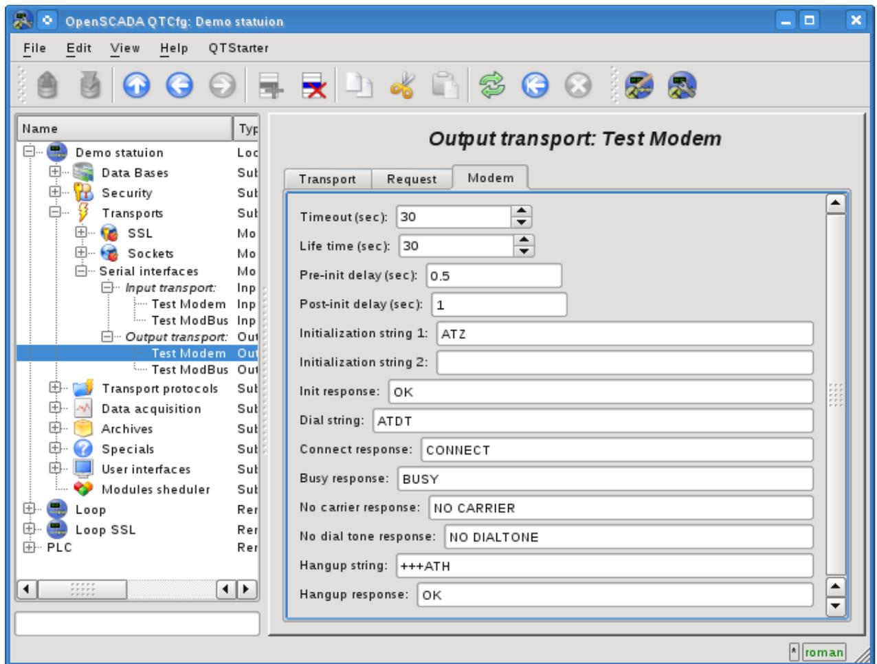
Fig.4. "Modem" tab of the configuration of modem of outgoing serial interface.
