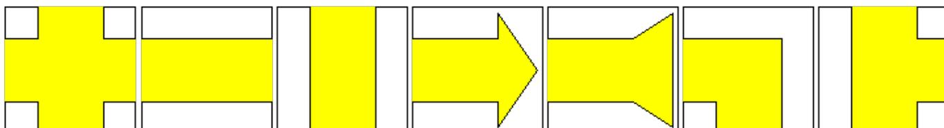
Fig.1. Elements of the pipeline from left to right: "Pipe-cross", "Line-pipe horizontal", "Line-pipe vertical", "Arrow", "Back arrow", "Pipe\_Ugol", "Pipe\_pipe-tee".
