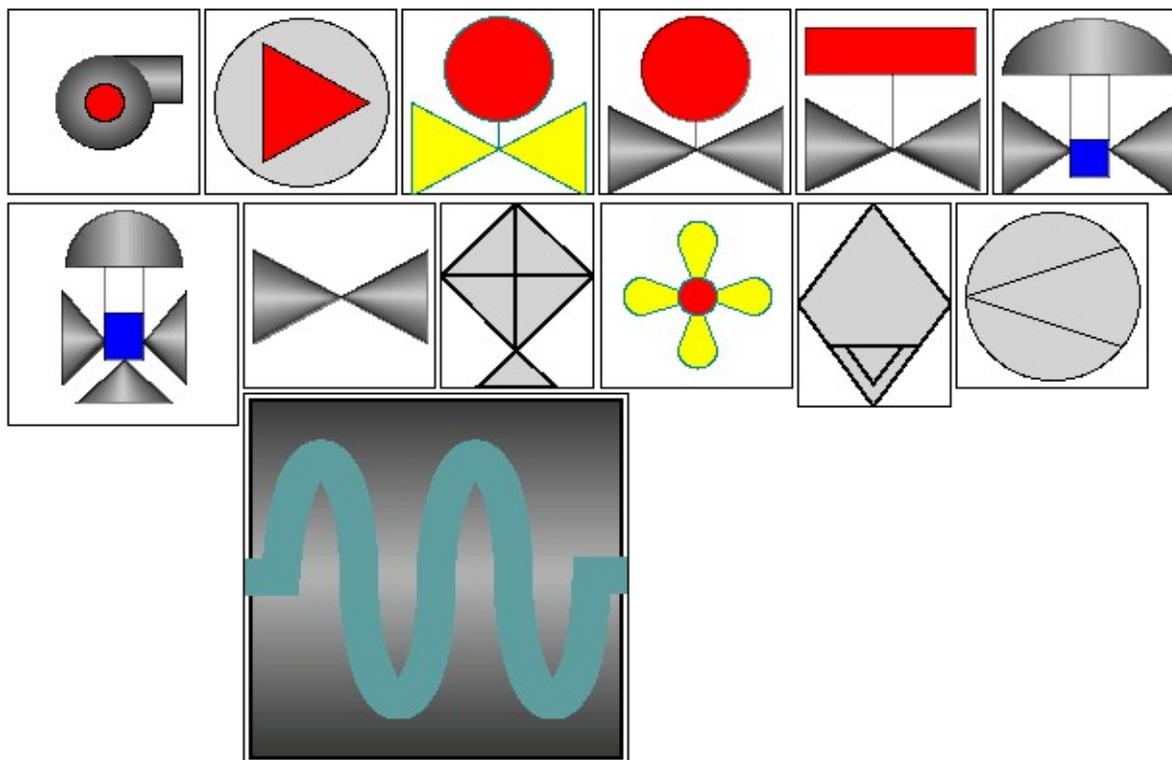
Fig. 1. Elements representing technological devices from left to right and top to bottom: "Compressor", "Compressor 1", "Bolt", "Crane", "Ball crane", "Crane and position", "Three-positioned crane", "Valve", "Cooler", "Cooler", "Separator", "Diaphragm", "Zmejev\_hor".
