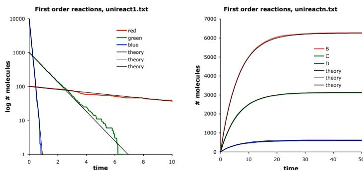
The panel on the left shows results from the configuration file `unireact1.txt`. First order reactions occur at rates that are in good agreement with theory over a wide range of rate values. The panel on the right shows results from the file `unireactn.txt`. Again, there is good agreement with theory.
