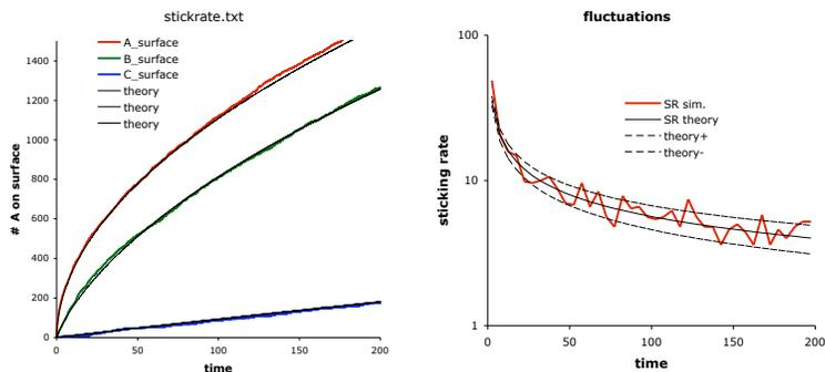
Results from example stickrate.txt, shown in red, are compared with the analytic solution for the sticking rate. The left panel shows the total number of molecules stuck to the surface. The right panel shows the average sticking rate with a 5 time unit averaging
