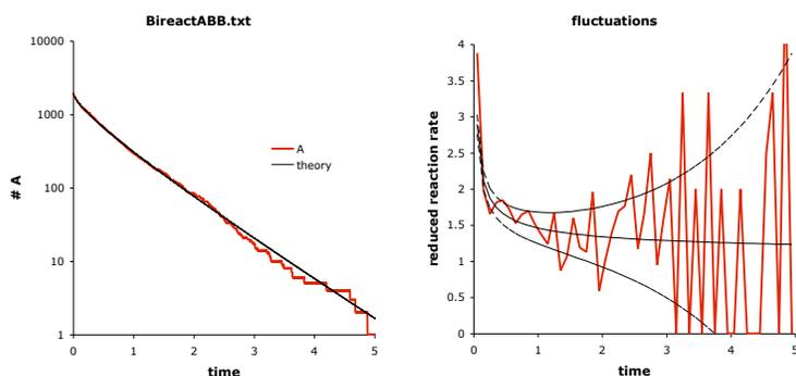
This example shows diffusion-limited bimolecular reactions from the configuration file bireactABB.txt, which simulates the reaction that is described in Figure 7 of Andrews and Bray, 2004. The left panel shows the number of surviving A molecules as a function of time with comparison to the time-dependent Smoluchowski equation. The right panel
