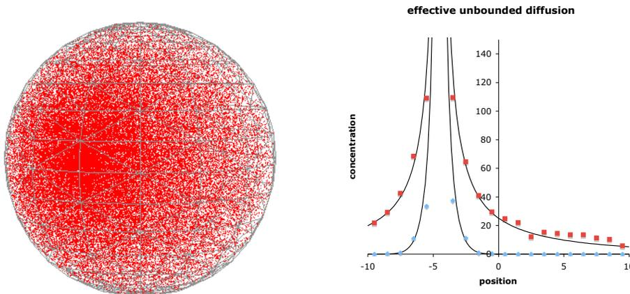
The left panel shows a snapshot from example emitter1.txt where it is seen that the emitter center is somewhat left of the sphere center and the sphere is triangulated. The right panel shows line profiles across the middle of the sphere, from (-10,0,0) to (10,0,0) at times  $t = 0.3$  s (blue) and  $t = 100$  s (red), with simulation data shown with points and theoretical results, from the equations above, in solid lines.
