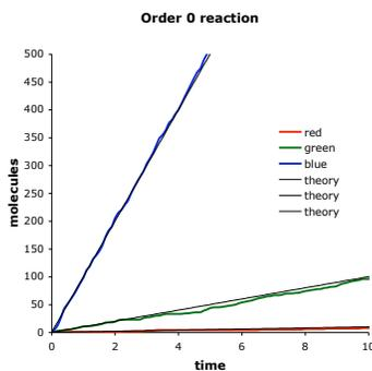
This shows zeroth order reaction molecule production with data simulated from the example file S8\_reactions/zeroreact.txt. Shown are the numbers of molecules produced as a function of time with three different production rates along with the deterministic theory for how many molecules would be expected.
